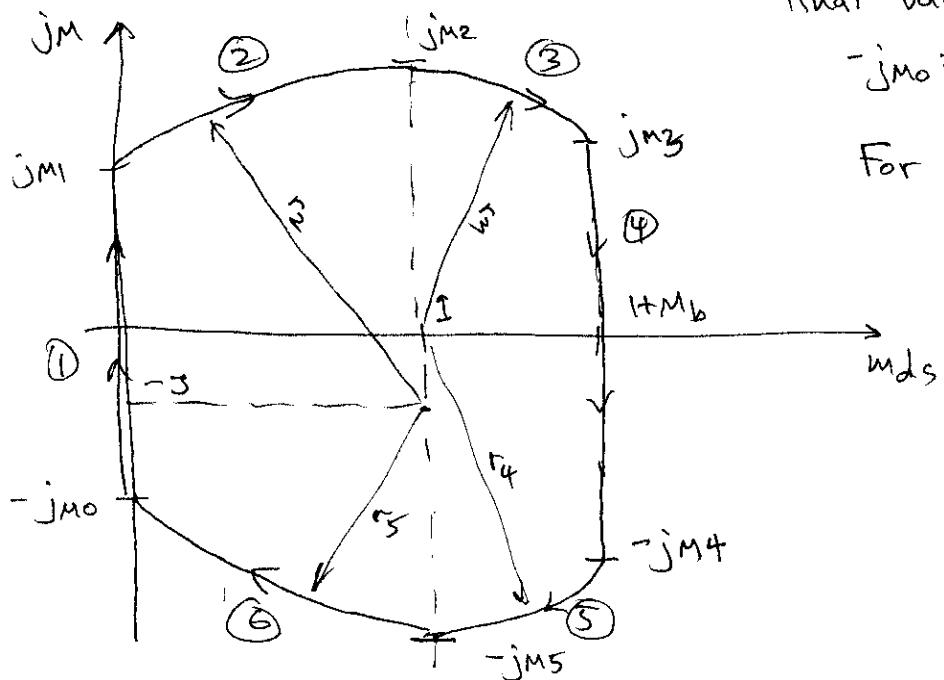
subinterval ⑥ length:  $\psi = \omega_0 t_6 = \tan^{-1} \left( \frac{1}{j_{M0} - J} \right)$
