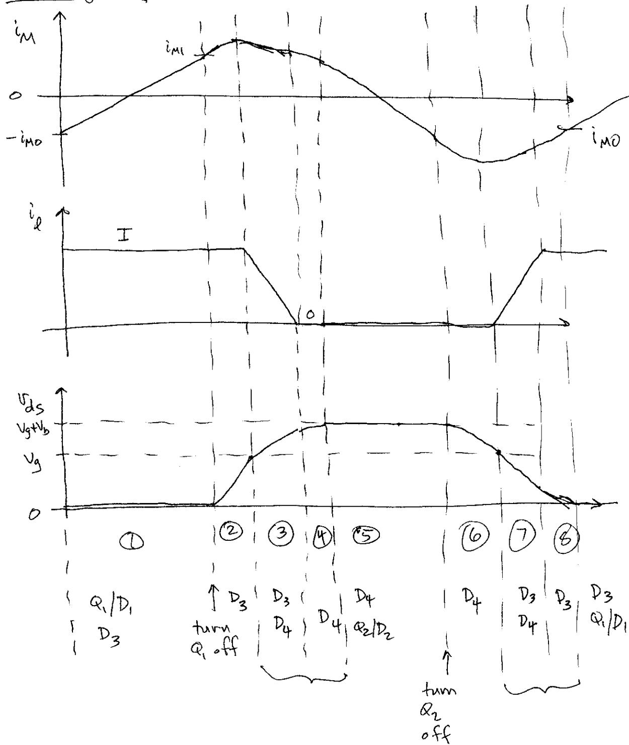
Several details can be changed, which technically lead to different modes of operation. Interval ③ can end either when  $D_3$  becomes reverse-biased by  $i_L$  reaching zero, or by  $D_2$  becoming forward-biased when  $v_{DS}$  reaches  $V_g + V_b$ . In either event both happen by end of interval ④. Similar discussion (in reverse) applies to intervals ⑦ & ⑧.
