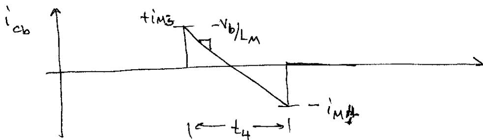
For the net charge to be zero, we must have  $i_{M3} = i_{M5}$ . By symmetry of the state plane trajectory, this also implies that  $i_{M2} = i_{M6}$
