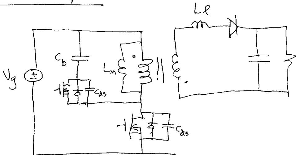
ZVT bridge example - snubbing the output diodes
