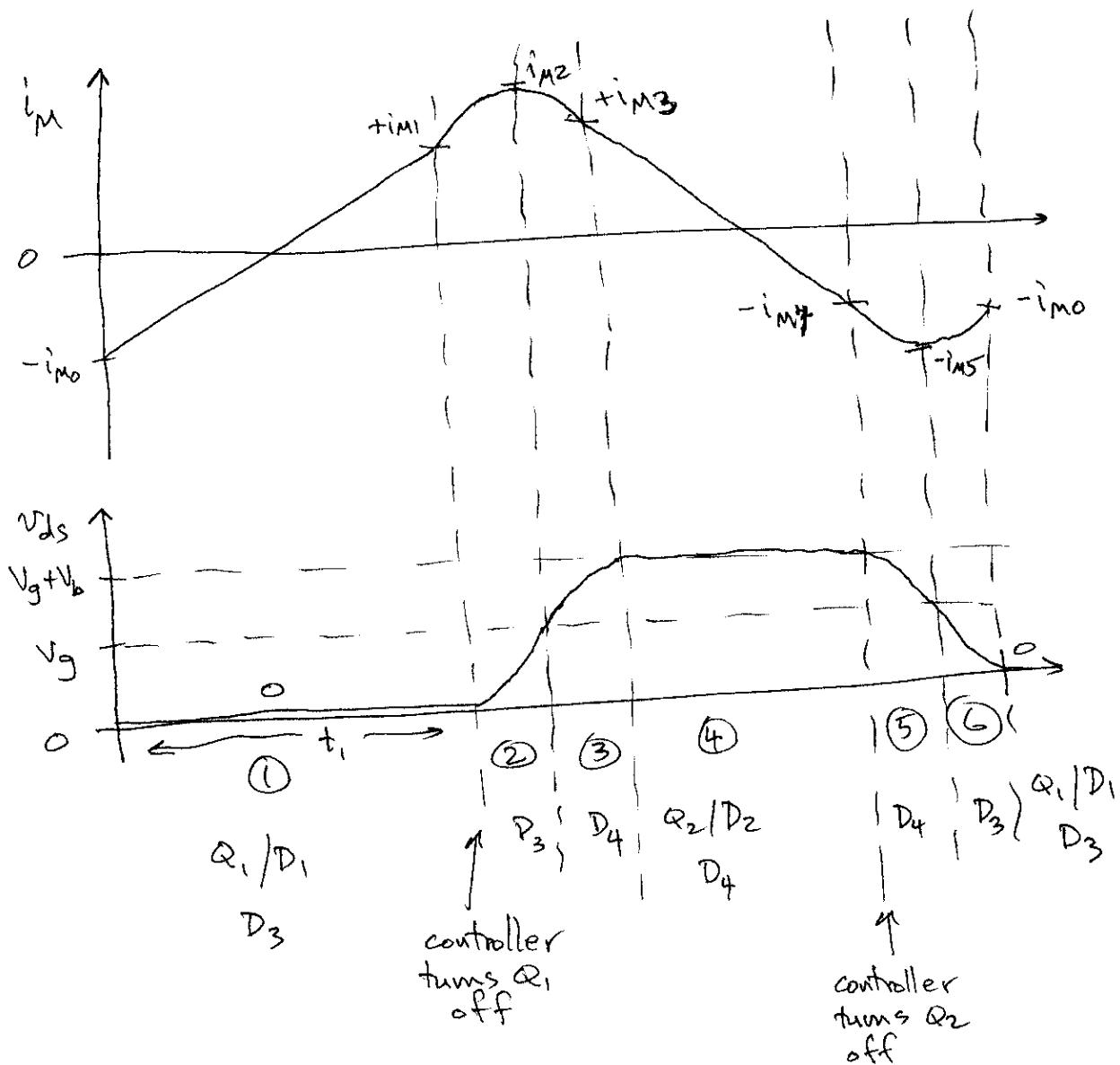
If we ignore  $L_e$ , then the model predicts that the load current  $I$  commutes instantly from  $D_2$  to  $D_3$  and vice-versa — secondary-side switching waveforms are idealized. But the primary-side switching behavior is modeled well. The predicted ZVS boundary is pessimistic.
