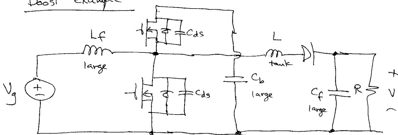
This can be viewed as a resonant switch network that employs an auxiliary switch. The two MOSFETs form a half bridge circuit
