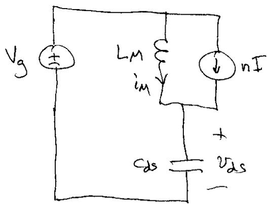
Note magnetizing current  $i_m$  must oppose reflected load current  $nI$  to discharge  $C_{ds}$ .
