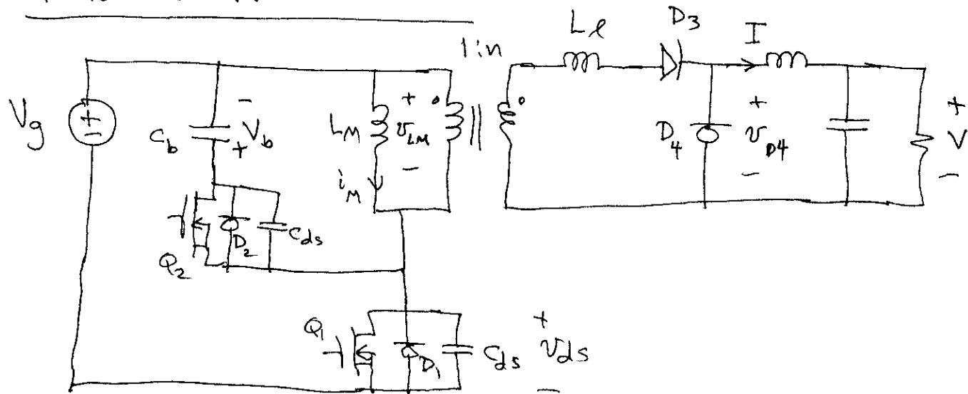
The auxiliary switch/active clamp circuit is used here to reset the transformer as well as to provide ZVS. The transformer is modeled with  $L_M$ ,  $L_E$ , and ideal L-N transformer. MOSFET output capacitances  $C_{DS}$  participate in ZVS. For the analysis below, we will lump both  $C_{DS}$  into a single effective capacitance in parallel with  $Q_1$ . Both  $L_M$  and  $L_E$  participate in operation of the tank.
