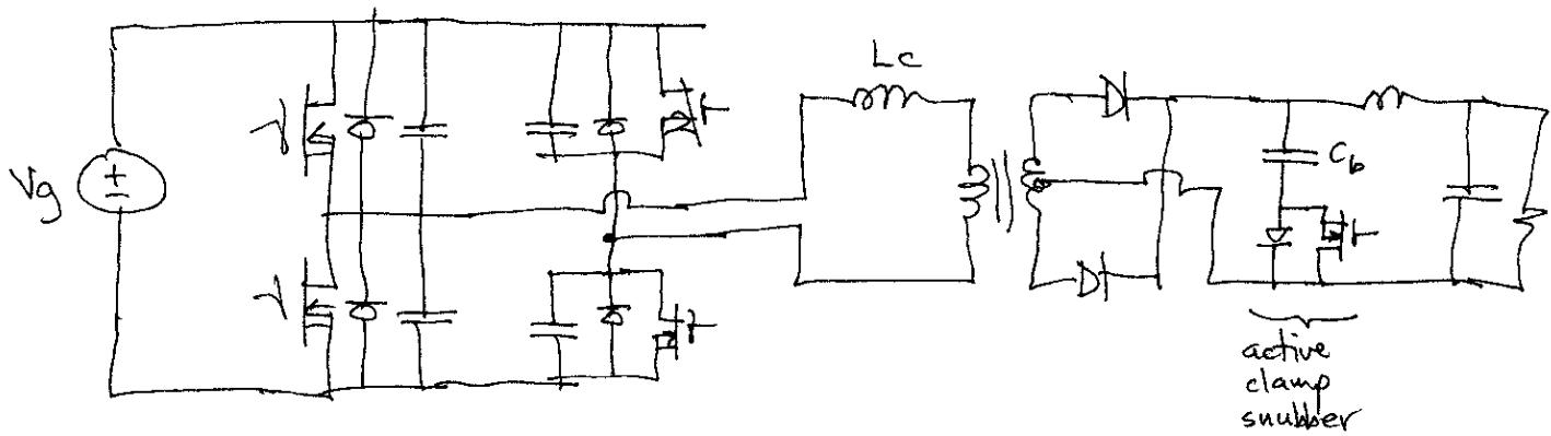
The above two applications can be viewed as improvements to the conventional dissipative voltage-clamp snubber
