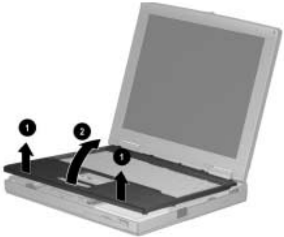
Figure 5-16. Removing the Top Cover
