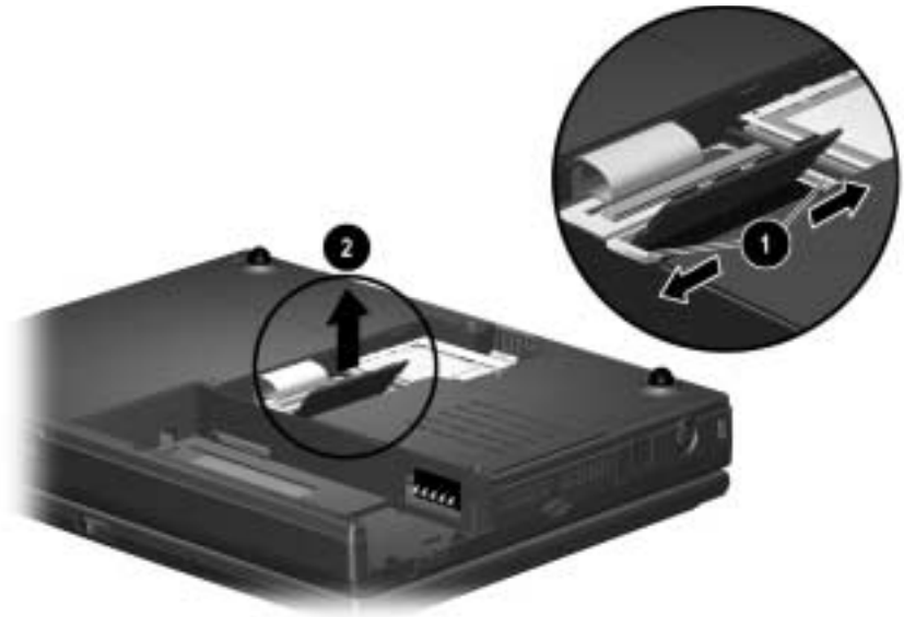
Figure 5-13. Removing a Memory Expansion Board
