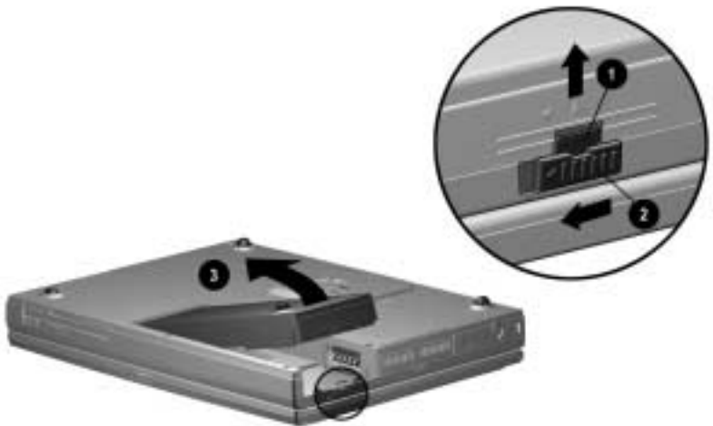
Figure 5-2. Removing the Battery Pack
