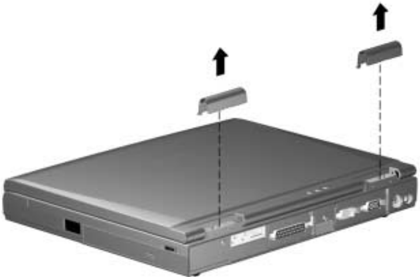
Figure 5-24. Removing the Hinge Covers
