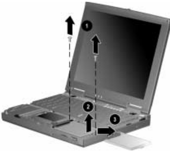
Figure 5-17. Removing the Hard Drive
