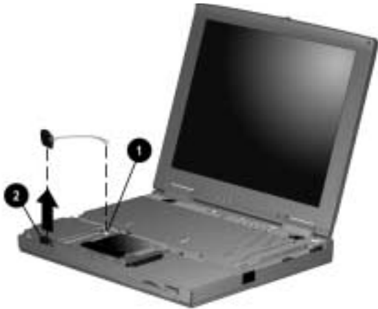
Figure 5-18. Removing the RTC Battery
