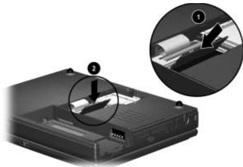
Figure 5-14. Installing a Memory Expansion Board
