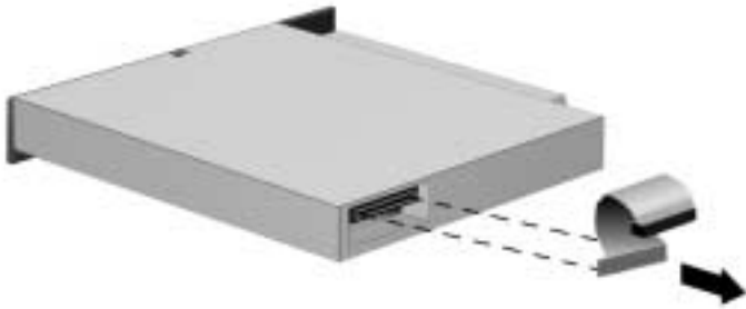
Figure 5-9. Removing the CD-ROM Drive Cable
