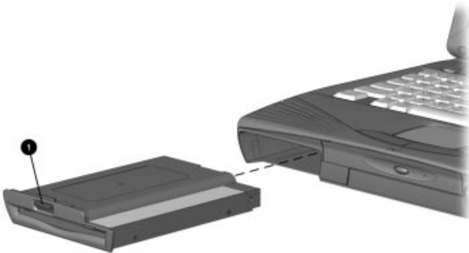
Figure 5-3. Removing the MultiBay Device
