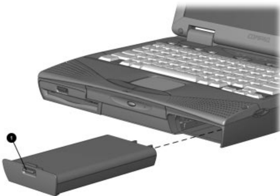
Figure 5-2. Removing the Battery Pack
