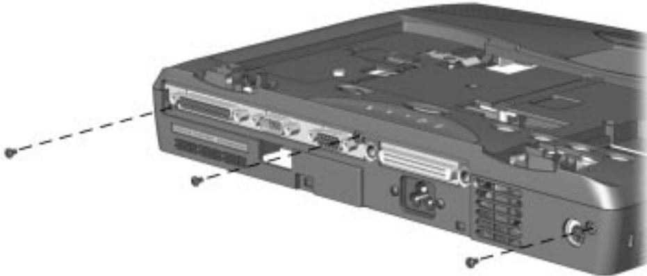
Figure 5-26. Removing the Top Cover Assembly Screws from the Back of the Unit
