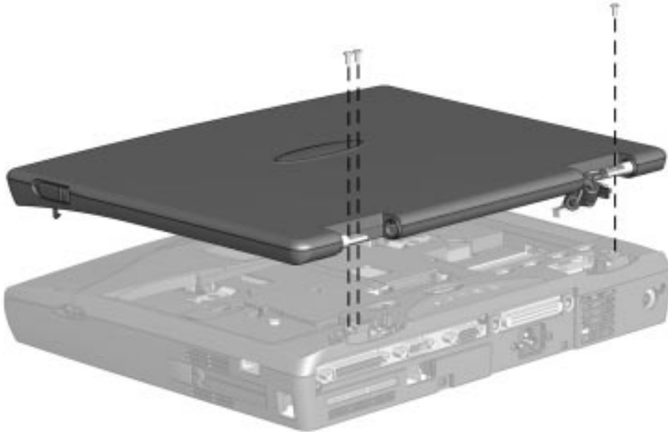
Figure 5-24. Removing the Display Assembly
