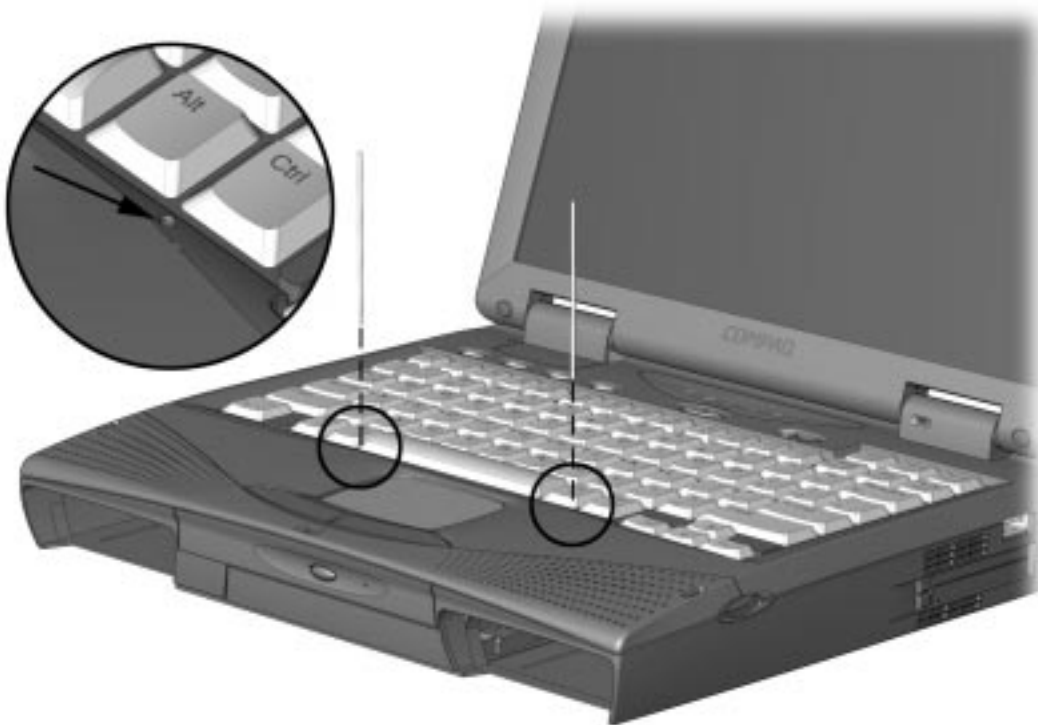
Figure 5-12. Releasing the Keyboard Latches
