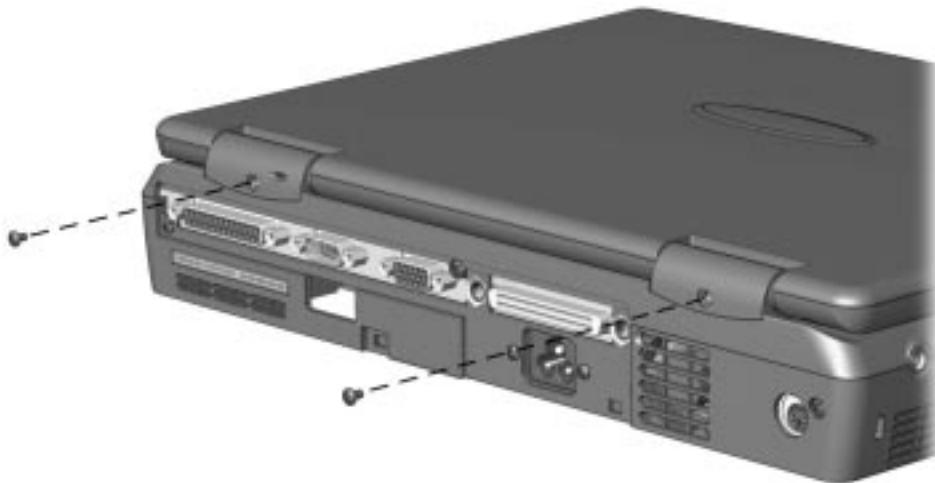
Figure 5-21. Removing the Hinge Cover Screws
