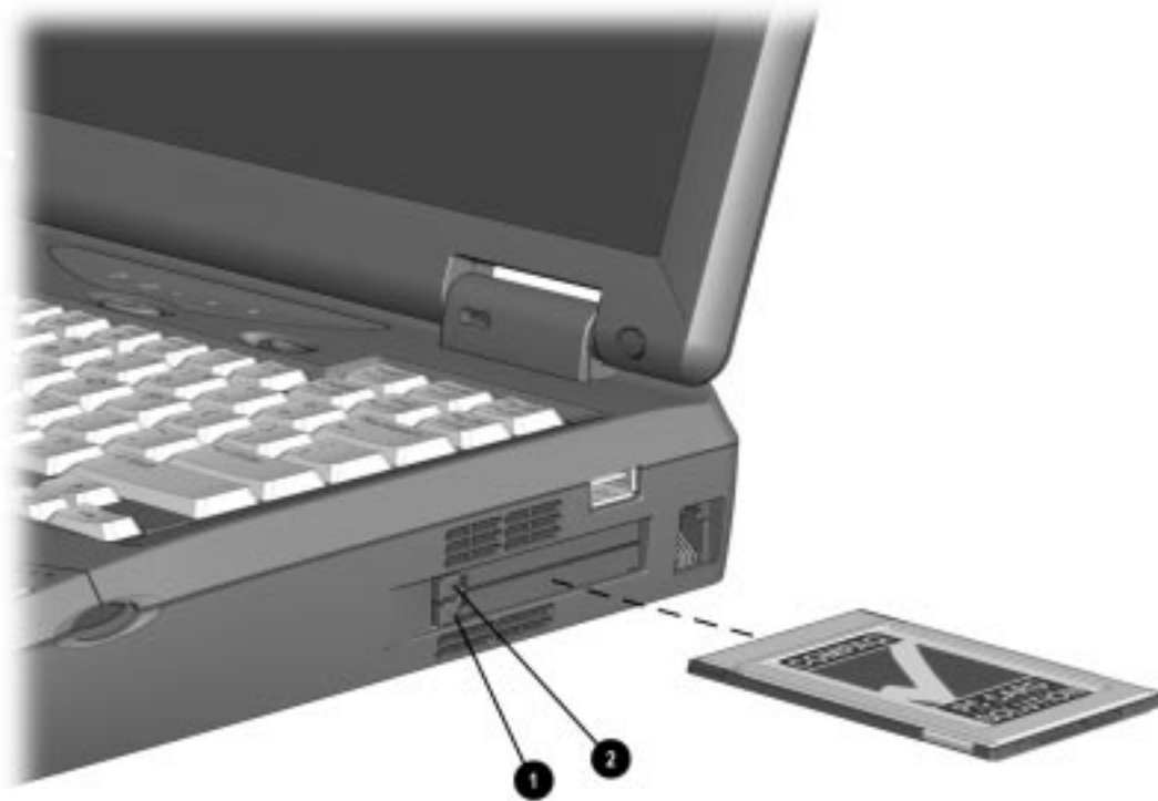
Figure 5-4. Removing the PC Card
