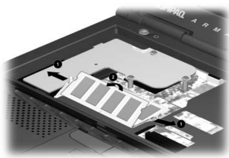
Figure 5-20. Removing a Memory Expansion Board
