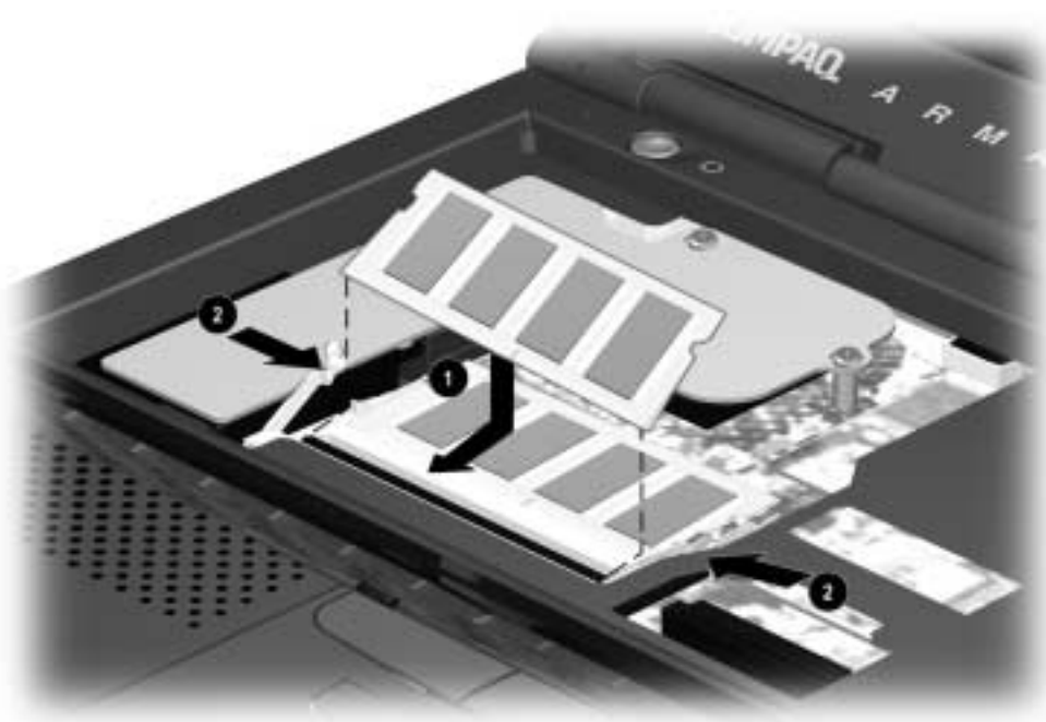
Figure 5-21. Installing a Memory Expansion Board
