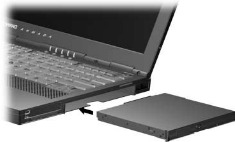
Figure 5-11. Inserting a Device into the MultiBay
