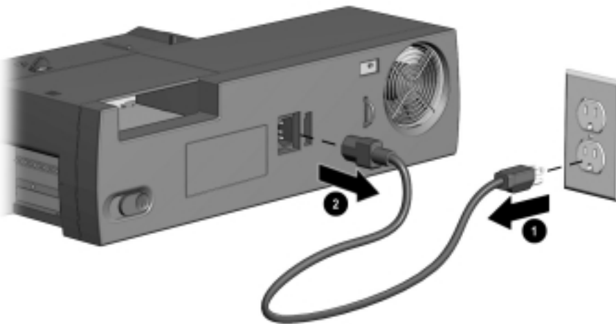
Figure 5-3. Disconnecting the Expansion Base
